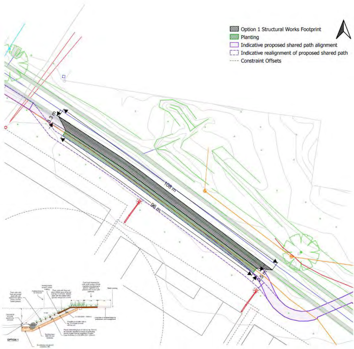
Figure 3 Upstream Section – Extent of Works
