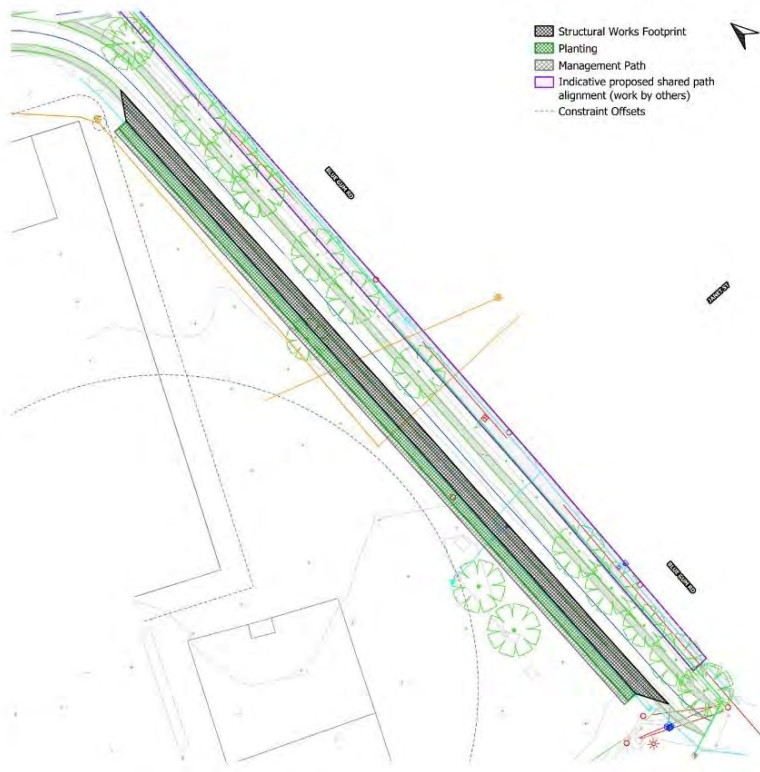
Figure 2-3 Concept design upstream plan of creek naturalisation works at Dark Creek, Heaton Park, Jesmond
