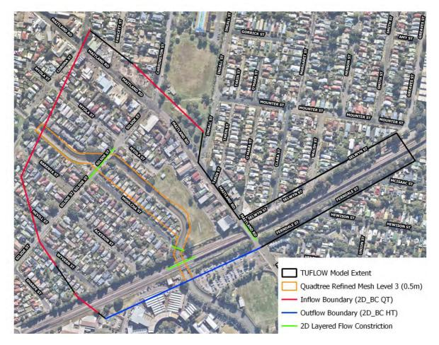
Figure 4-4 TUFLOW Model Setup
