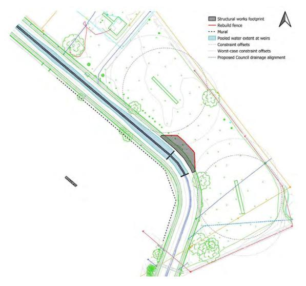
Figure 2-2 Concept design plan of creek naturalisation works at Throsby Creek, Litchfield Park, Mayfield
