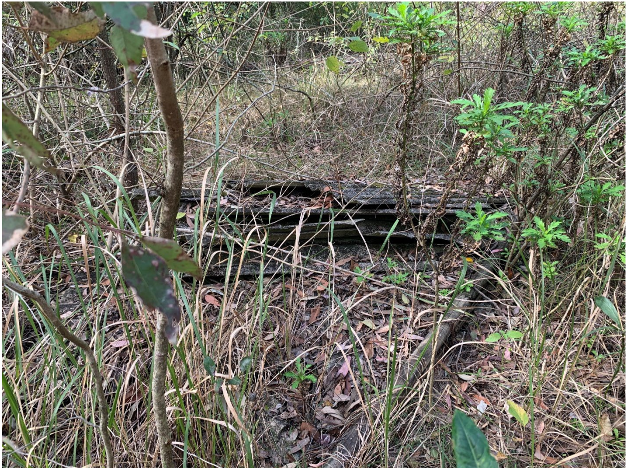
Photograph 1: Corrugated asbestos containing fibre cement sheeting
